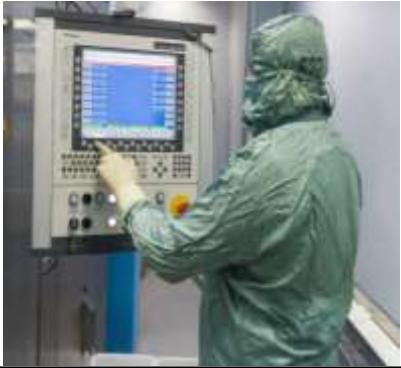
Rommelag 321 BFS Machine Multi-dose filling (3000 bottle/hr) It fills 5 ml, 10 ml and 15 ml sterile ophthalmic solutions.
