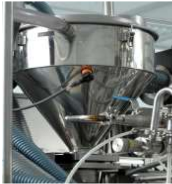
Rommelag 321 BFS Machine Multi-dose filling (3000 bottle/hr) It fills 5 ml, 10 ml and 15 ml sterile ophthalmic solutions.
